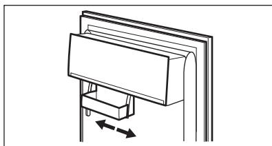
This model is equipped with a variable storage box.
